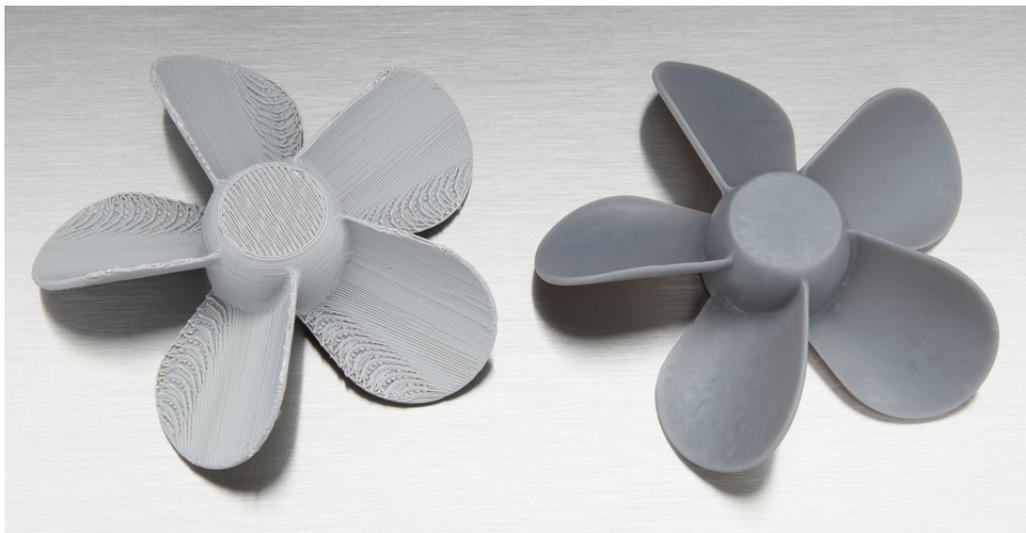
*Figure 3 – a fan blade printed by two types of 3D printers. Left: filament (FDM) printer, Right: resin (SLA) printer*
